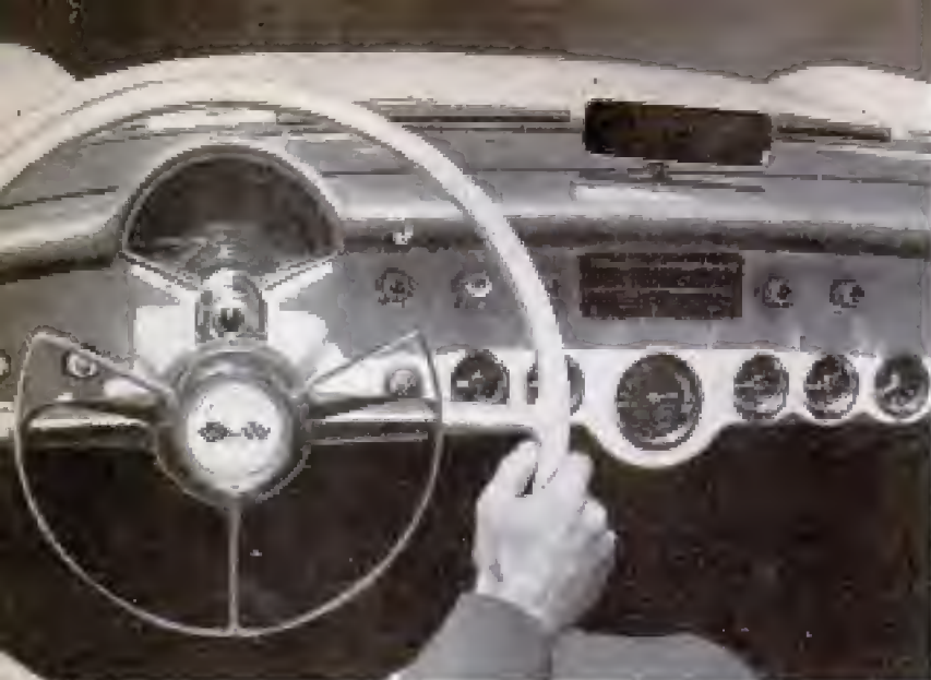
Dash is poorly arranged, say some owners, with tachometer and other dials placed too far to right for easy reading
